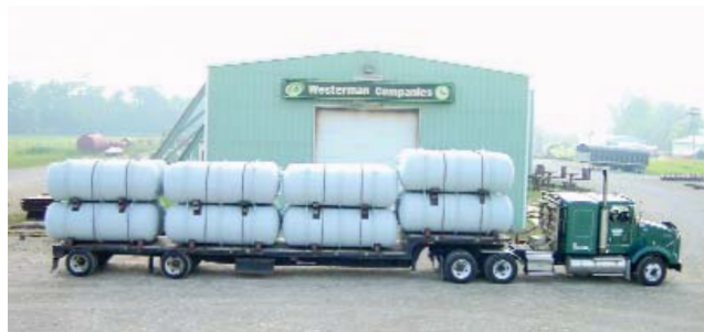
A truck loaded with "48G" UF 6 cylinders leaving Westerman Companies for delivery to a customer.
