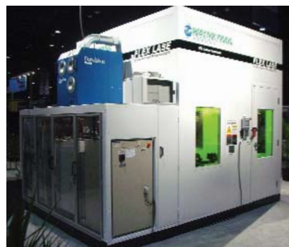
Universal laser processing cell, which is used for laser welding
