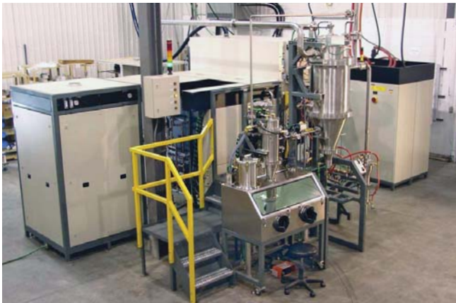
Buckeye Silicon's Reductive Combustion Process (RCP) manufacturing system
