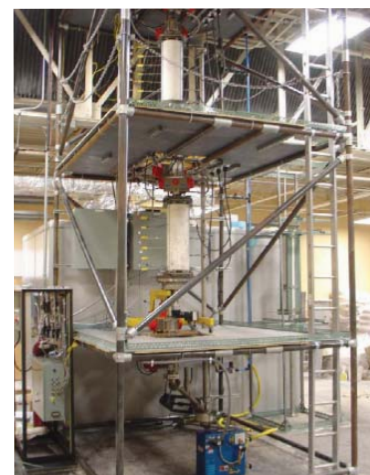
OSU sub-pilot scale (25 kWth) SCL unit. The proposed pilot plant is a 10 time scale up from the sub-pilot unit shown above.
