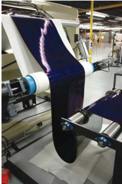
Xunlight's coated amorphous silicon solar cell material off of the front-end production line.
